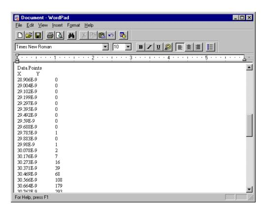
You have just copied the current marker and statistical data, as well as the histogram bin values (X values) and their corresponding counts (Y values) between the current markers to the "WordPad" word processor. You may need to scroll the display down to see all of the statistical and histogram data. This type of information could also be shared with a spreadsheet program.
