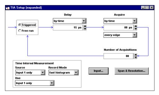
This is the TIA setup menu to make data-to-data measurements on the drive under test. The screen is configured as a flow diagram showing the various stages of the measurement. Reading from left-to-right you can see that the TIA will wait for a trigger, delay 15 µs and then measure every edge for 80 µs. This sequence is repeated 80 times, which results in the acquisition of 80 consecutive sectors.
