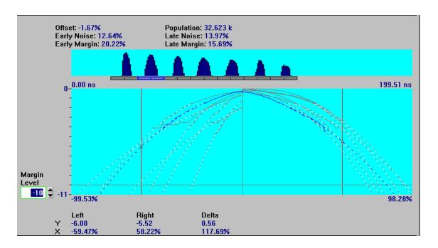
This display now shows the window margin curves for the individual distributions overlaid, rather than combined. One segment beneath the histogram is highlighted (in blue). Its corresponding window margin curve is also highlighted in blue on the main display. The window margin results and the marker readouts correspond to this selected segment.
