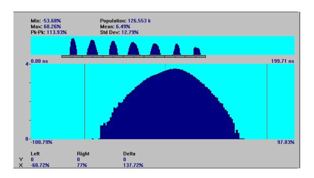
This result display allows you to analyze histograms by defined "segments" or decode windows. The panorama display shows the individual distributions as with the previous histogram display, but the main display shows the histograms combined, or added together based upon the segment definition. Notice the darkened grid beneath the panorama display. This represents the currently defined segments. The half tic mark represents the center of each segment.
