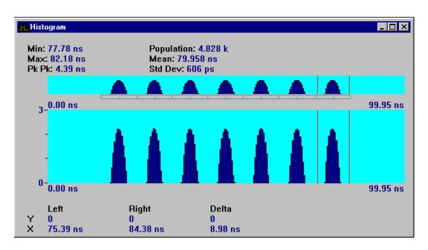
Now you can read the statistics for one distribution. The panorama display (the display just below the statistics) always shows the entire span of the histogram, while the main display below can be scaled to show a closer view of the data.
